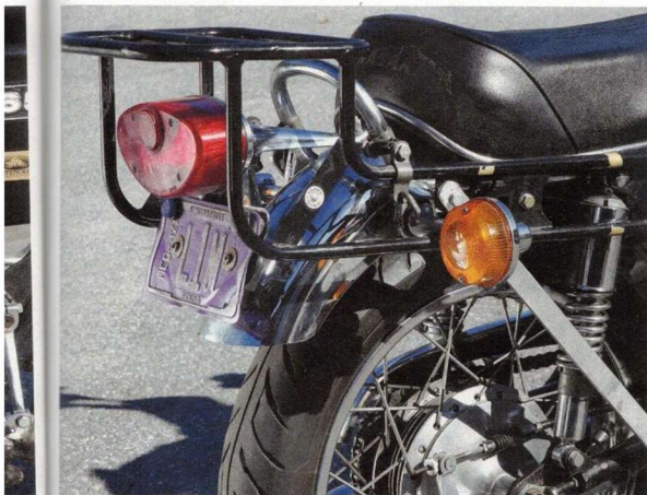
The W3 has been upgraded with modern Avon Roadrider tires, quartz lighting, and new Hagon shocks at the rear.
