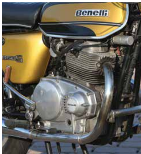
Above: With British competitor 736cc Rickman Enfield Left: Short-stroke ohv twin was one Italian take on what British twins should have become
