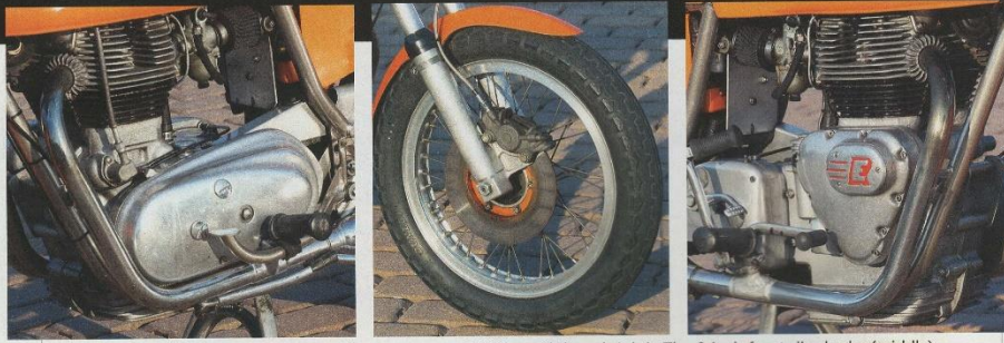
The 736cc air-cooled twin makes 52.5 horsepower at 6,500rpm (left and right). The 8-inch front disc brake (middle).
