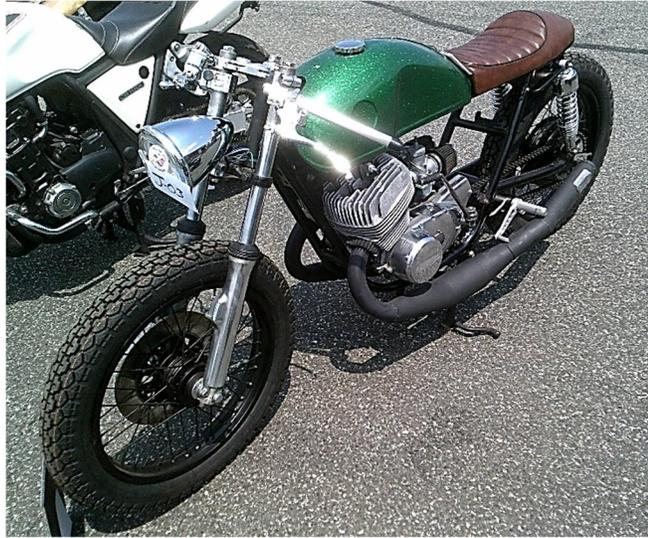
Right: a Suzuki T500 project with expansion chambers; *surely an extreme environmental hazard/smoking racket.*
